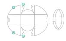
1 INSERT STRAP THROUGH EITHER TOP HOLE & SNAP TO CREATE LOOP
